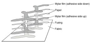
Figure 6: Inflation channel layers heat-sealed in fabrication
